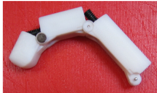
Fig. 3. The first fabricated device. Note some design changes noted in the text from Fig. 2 are visible here. The dark circle on the distal-medial hinge axis is the hall effect sensor magnet. The black rods are attached to motor shafts for clarity.
