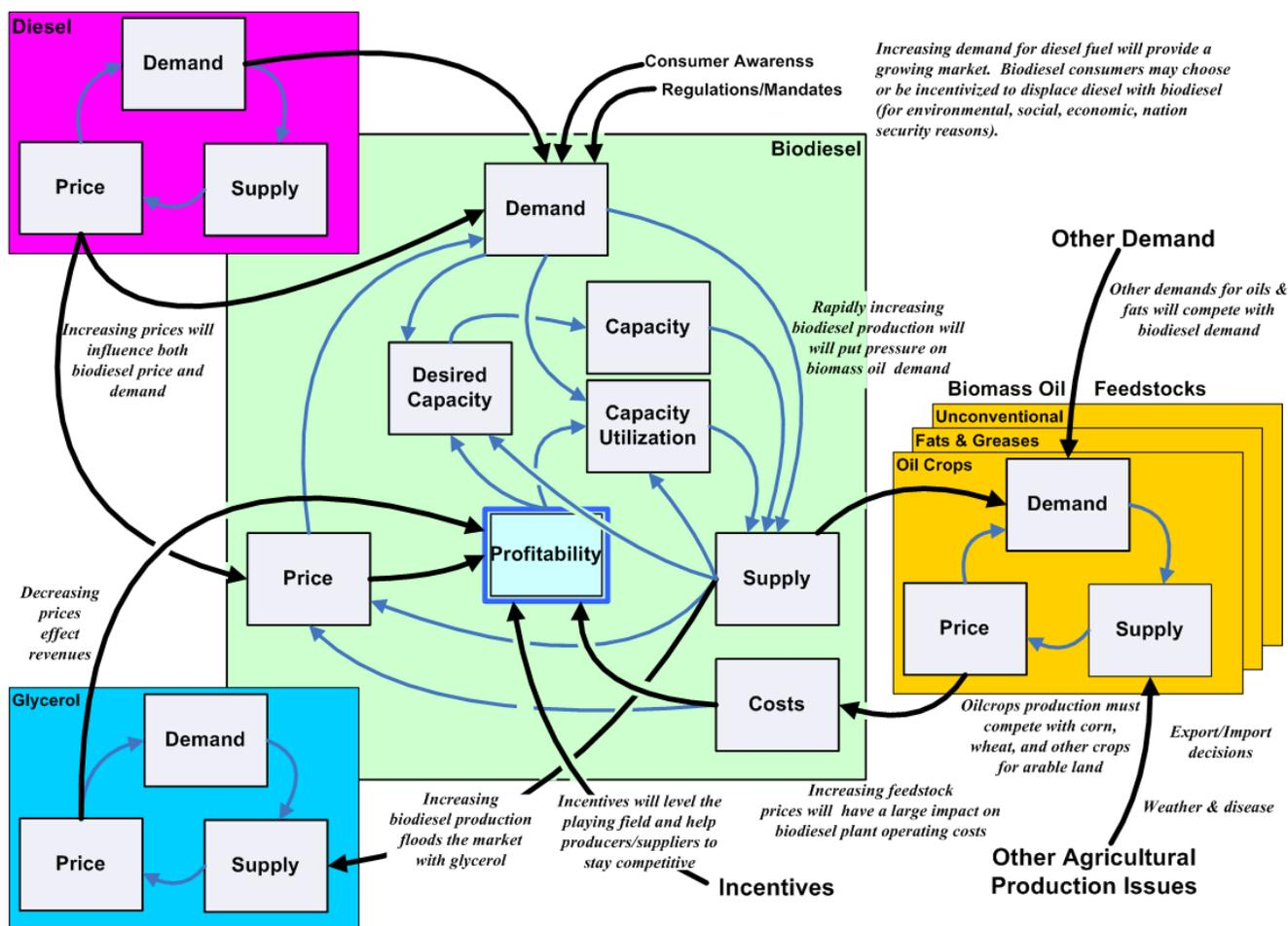
Fig. 4. Biodiesel Market Overview Diagram shows the interconnections between biodiesel and other markets-diesel, biomass oil feedstocks, and glycerol
