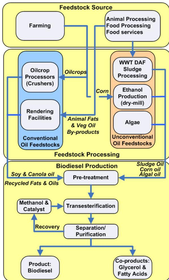
Fig. 2. Biodiesel Production Process and Feedstock Sources
